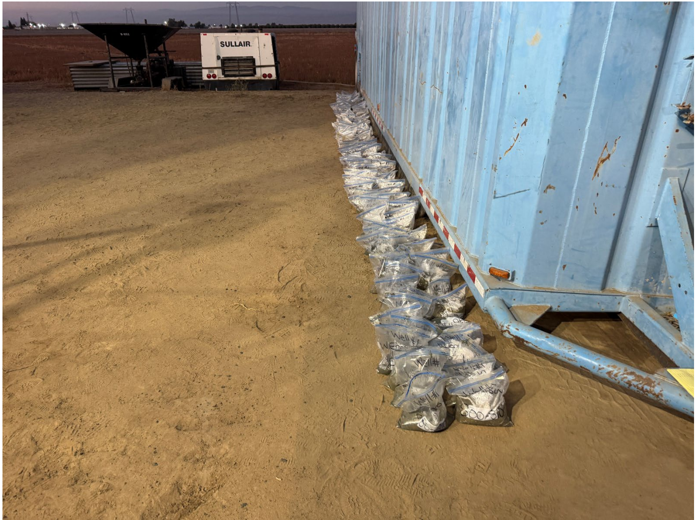
Drill Cutting Samples
